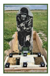
A lightweight steel frame, the AC120 accommodates both, the M3200M Pop-Up and LOMAH H-Bar for portable applications.
