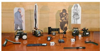
Target mechanism units and distraction devices can be activated from trigger devices, such as pressure mats, PIR sensors, etc causing a target mechanism unit to turn to a Shoot or No Shoot exposure. The setting up and changing of a range layout is easily achievable as communication between the target unit, trigger devices and distraction units is via radio, eliminating the need for trailing cables.
