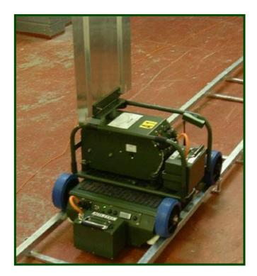
Carrier with a M2100M held by two Quick fit connectors
