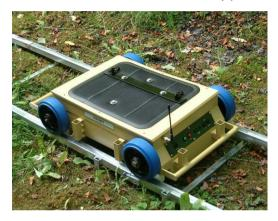
The armour panel support bracket fits into the two location tubes, when specified. Option for advancing target is also catered for with location tubes at one end.
