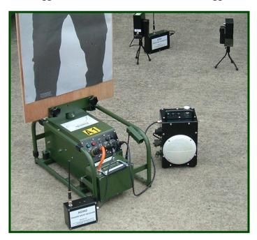
The training program may be initiated by the action or movement of the trainees as they advance through the range - e.g. opening of a door which in turn breaks an infra red beam, simultaneously activating a target to turn and a sound (e.g. shouting).
