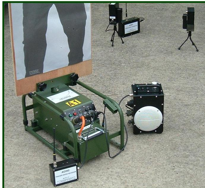
The training program may be initiated by the action or movement of the trainees as they advance through the range - e.g. opening of a door which in turn breaks an infra red beam, simultaneously activating a target to turn and a sound (e.g. shouting).
