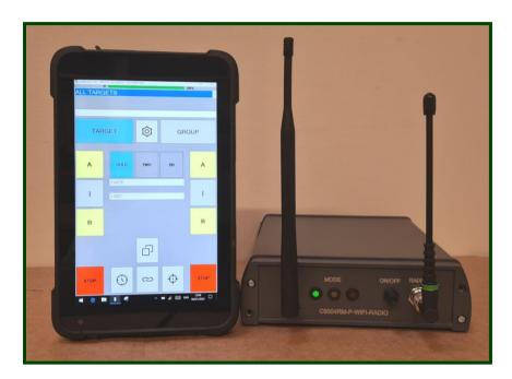
The C9800M Tablet Range Controller is a user-friendly handset designed for both left and right-handed operators, on indoor and outdoor ranges.
