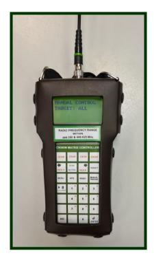
The C9090M MATRIX handheld controller has been developed to enable the training officer to have direct control over live fire close combat training exercises.
