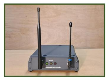
The C9004RM acts as an Interface between the PC and C9800M Tablet Controller to the target mechanisms units.
